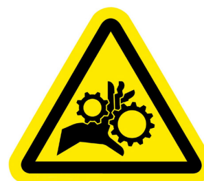
Figure 11: Gear Pinch Point
